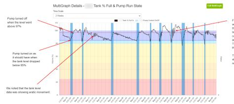
From the data collected from this tank, we identified a problem. After inspecting the site, it was found that the bladder lining the tank was leaking, which was causing fluctuations in the tank level. It also resulted in levels rising above 97%. The varying pump run times also indicated that there was an issue with the tank.
