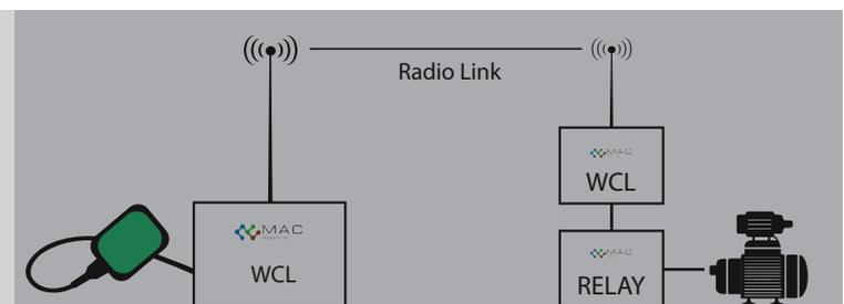
*When the float switch in the water tank hits the low level setpoint, an on command is sent to the pump via radio. When the water tank level hits the high setpoint, a stop command is sent to the pump via radio*
