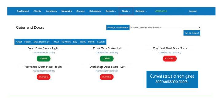
Using radio telemetry connection to position sensors, this solution provides remote information on the position of gates and doors. Alerts can be raised when gates and doors are opened with dates and times recorded.
