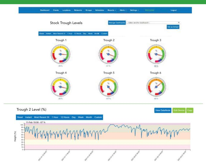
Radio telemetry unit reading water level sensor in troughs. Data from radio monitoring sites requires a gateway that connects to the internet via 4G, Provides remote data of water level in troughs with graphical history of data and email and/or SMS alerts on specified levels. This solution is designed for applications where there are multiple monitoring sites that are within radio range of the gateway.
